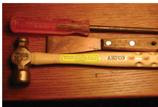
FIGURE 1. Copper-beryllium alloy tools with instructions for grinding to maintain chamfer
